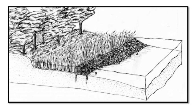
Figure 38. Example of bioengineered shoreline restoration techniques. A) Rock rip-rap in combination with plantings. B) Willow bundles or coco coir logs in combination with plantings.
