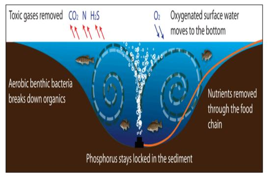
Figure 25. A diagram showing the laminar flow aeration mechanisms. ©RLS
